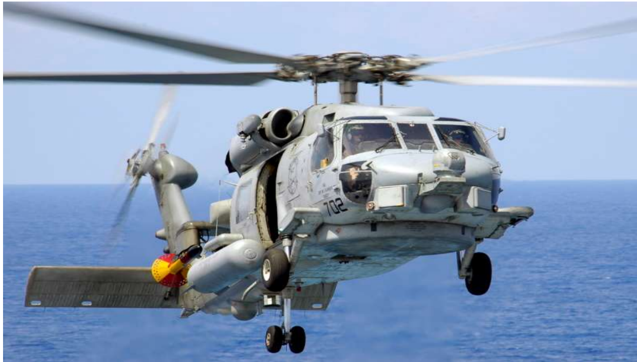
Figure 3. U.S. Navy MH-60S Seahawk helicopter engaged in airborne mine countermeasures operations. Helicopter-based systems enable standoff detection and neutralization, though their effectiveness is constrained in high-threat littoral environments.
