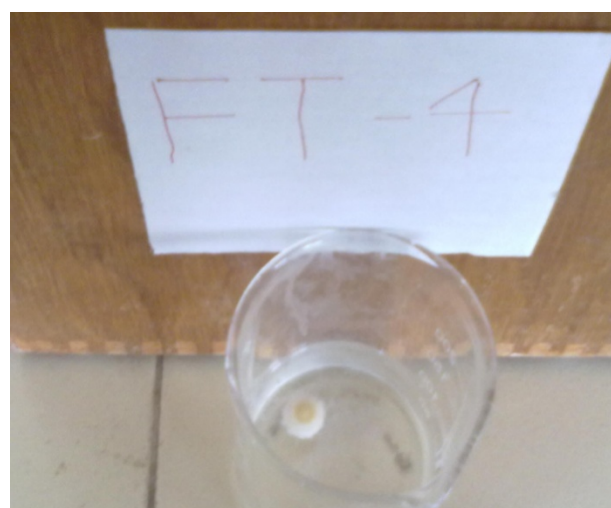
Fig 1: In-vitro buoyancy study of formulation FT-4 (Time 0 sec to 24 hours)
